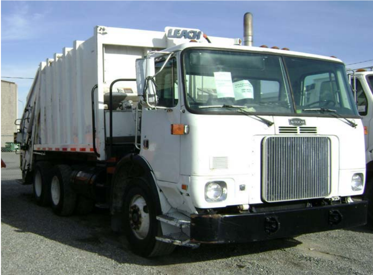
SWS 6324 2004 Autocar ExpeditoR w/ Leach Alpha 20yd Rear Loader
